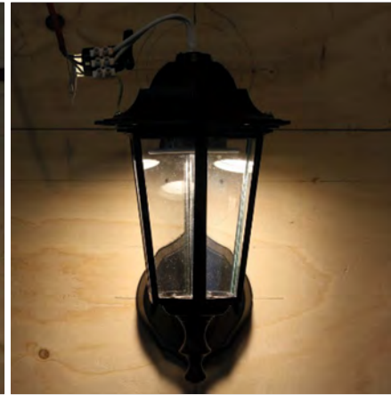
▲ Fig. F9: GU10 downlight holder fixed in canopy.
