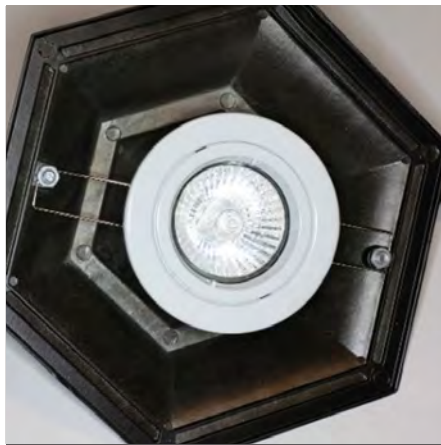
▲ Fig. F10: Luminaire experiment. Domestic GU10 downlighter unit replacing original lampholder.
